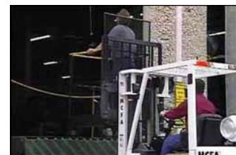
Figure 107. Specialized platform for lifting coworker. Note: There is a guard on the back of the platform to keep the person in the platform and protect the worker's arms and hands.
