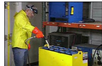
Figure 12. Water is added at the end of the charge by operator wearing PPE.
