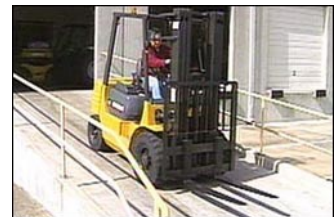
Figure 115. Traveling down ramp without load.
