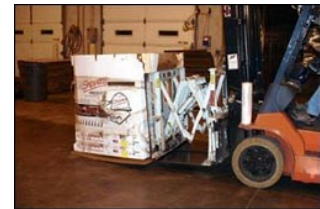
Figure 22. Slipsheet attachment eliminates need for pallets.
