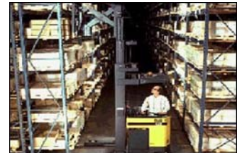
Figure 16. Triplex mast in narrow aisle rider reach truck. Note that the forklift is removing stock from a rack. Foot and truck traffic in the opposite aisle way should be controlled to prevent injury from falling materials.
