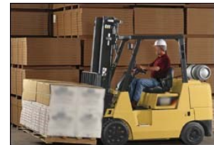
Figure 74. Operator traveling with load lowered.
