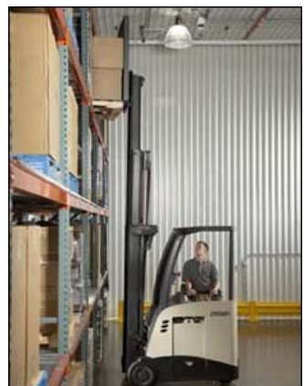
Figure 101. Ensure adequate overhead clearance.
