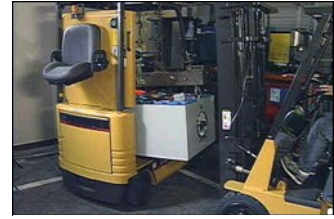
Figure 8. Battery hoisted from forklift compartment with
