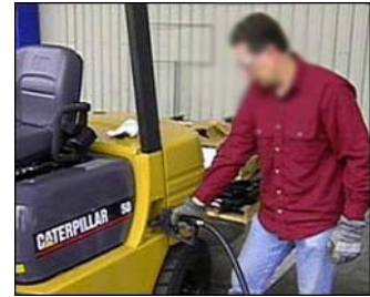
Figure 2. Operator refueling diesel-powered forklift.
