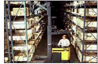
Figure 121. Reach truck with pantograph attachment that scissors forward from the mast to retrieve the pallet.
