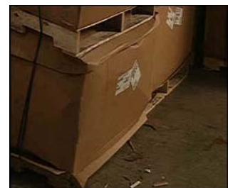
Figure 80. A damaged carton is an unsafe load to carry.
