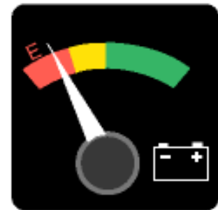
Figure 6. The battery charge gauge indicates over-discharging.
