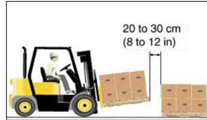
Figure 82. Operator stops slowly in front of the load platform.
