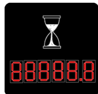
Figure 38. Hour meter indicating the total time the forklift has been in service.
