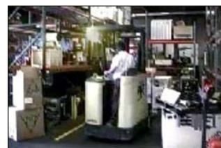
Figure 69. Warning strobe light flashing as operator backs up.
