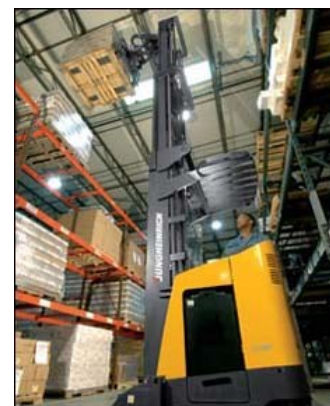
Figure 15. Reach truck with mast extended.
