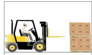
Figure 83. Operator lifts load with the mast vertical.
