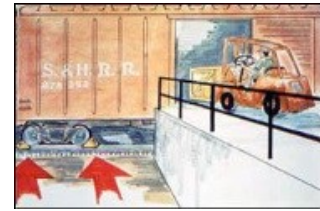
Figure 93. Use positive protection to prevent railroad cars from being moved.
