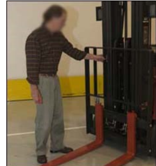
Figure 54. Operator inspecting the load backrest as part of the pre-operation inspection.
