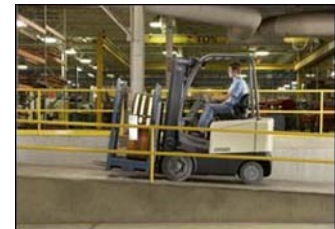
Figure 109. Drive loaded trucks forward going up a ramp.
