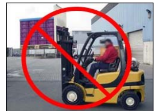
Figure 75. Do not travel with the load elevated.
