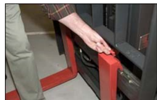
Figure 51. Operator inspecting the top clip retaining pin for the forks.
