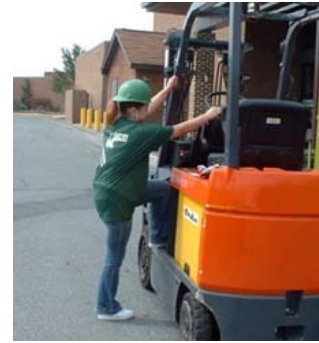
Figure 62. Operator grasping hand grips when mounting the vehicle.
