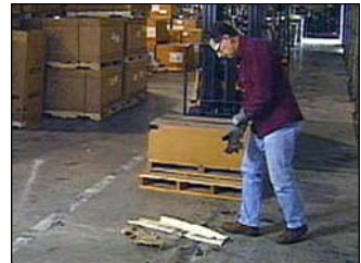
Figure 99. Get off the forklift and remove the obstruction.
