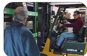
Figure 108. Operator signaling to coworker to stand back.
