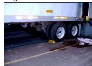
Figure 92. Wheels are chocked prior to boarding.
