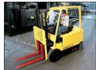
Figure 110. Traveling down ramp without load.
