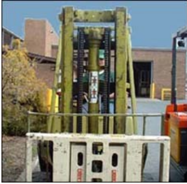
Figure 17. Mast with central cylinder
