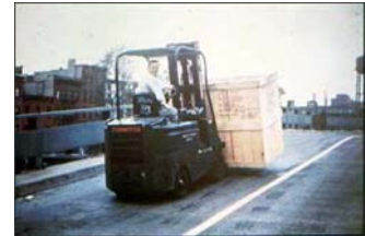
Figure 113. Traveling down ramp with a load.
