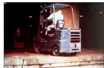
Figure 116. Always look in the direction of travel. Be careful at the edges of the loading docks.
