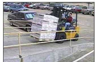
Figure 112. Traveling up ramp with load.
