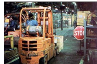
Figure 64. Stop signs posted to regulate traffic flows.
