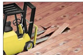
Figure 100. Forklift weight exceeded the load limit of the flooring.
