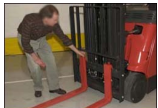
Figure 50. Operator checking condition of the forks.
