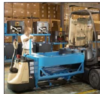
Figure 7. Electric forklift properly positioned while changing battery.
