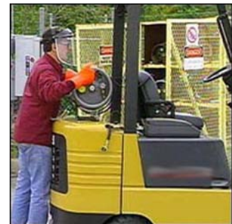
Figure 3. Operator changing LPG container.
