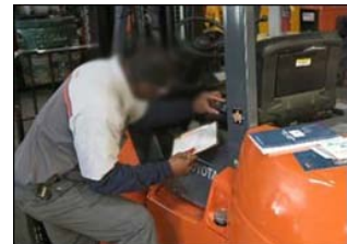
Figure 53. Operator checking the seat belt as part of the pre-operation inspection.
