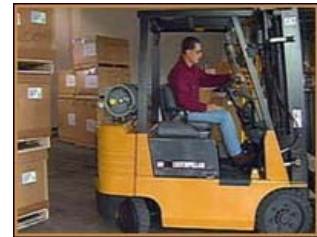
Figure 71. An exaggerated tail swing is caused by rear wheel steering; the operator is turning left and the rear is swinging toward the right.
