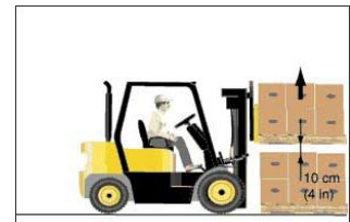
Figure 87. Operator is lifting the load.
