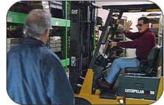
Figure 102. Operator cautioning pedestrian to stop.
