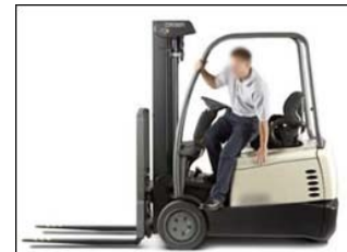
Figure 63. Operator dismounting a forklift.
