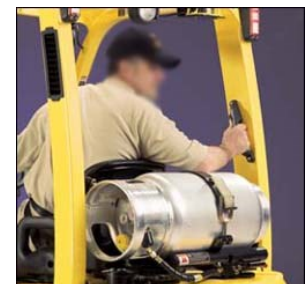
Figure 73. Operator looking in the direction of travel and keeping arms in the confines of the vehicle.
