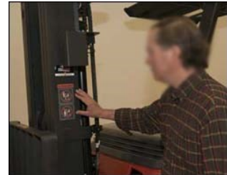
Figure 52. Operator ensuring that warning decals are in place and legible.
