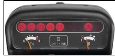
Figure 32. Dashboard showing gauges on a forklift.
