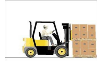
Figure 86. Operator slides the forks into the pallet until they are fully under the load.
