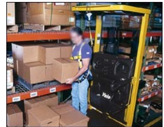
Figure 122. Order picker operator using full body harness.
