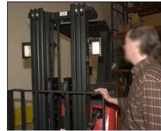
Figure 57. Operator performing operational inspection of working lights.
