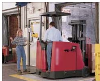
Figure 118. Paint the edges of loading docks to improve visibility. Check for pedestrians, over vehicles, and other obstacles when exiting trailers.
