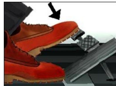
Figure 31. Operator depressing inching pedal.
