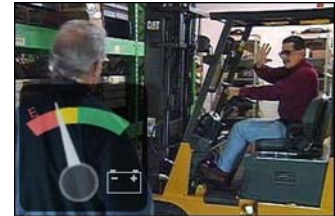
Figure 11. Discharging a battery beyond the manufacturer's recommended discharge level over works the battery making recharging more difficult and may damage or ruin the
