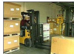
Figure 65. Operator slows down and sounds the horn at cross aisles where vision is obstructed.
