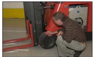
Figure 49. Operator checking condition of tires.
