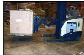
Figure 89. Reach trucks maximize maneuverability in narrow aisle.
