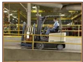
Figure 72. Drive loaded trucks forward going up a ramp.
