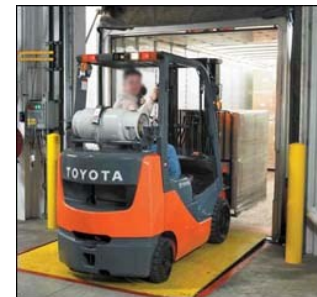
Figure 94. Operator using warning light and looking in the direction of travel when exiting a truck trailer.
