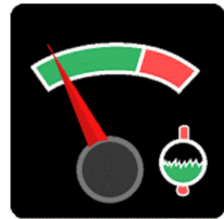
Figure 35. Engine temperature gauge in the normal zone.
