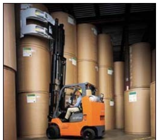
Figure 24. Forklift equipped with a barrel clamp attachment.
