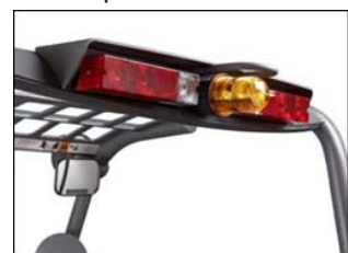
Figure 46. Warning strobe light flashes as operator backs up.
