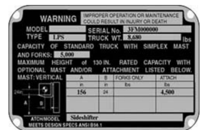
Figure 27. This data label indicates that this forklift has a 156" upright mast height in column A and a 24" load center in column B. Its stated capacity is 5,000 lbs with just its forks. With the sideshifter attachment, its stated capacity is 4,500 pounds. The truck weighs 8,600 pounds.
