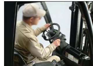
Figure 58. Operator conducting operational inspection with engine running.
