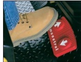
Figure 70. Using pedal to shift from reverse to forward.
