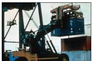
Figure 25. Reach stacker used in marine terminals and longshoring.
