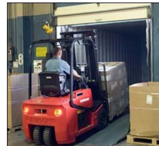
Figure 95. Entering a truck trailer with adequate overhead clearance.
