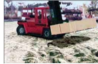
Figure 98. Maintain contact with ground by crossing uneven areas at an angle.
