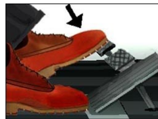
Figure 68. Operator is releasing the inching pedal, setting the direction control to forward and pressing the accelerator. (The brake is the middle pedal.)
